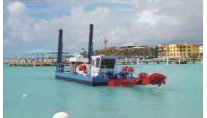
Nil Diyawara Cutter Suction Dredger
