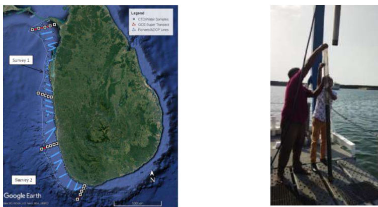
Figure 11. Overview of survey tracks consisting of transects lines (left) utilizing Vibro-corer for sea bed measurements (right)
