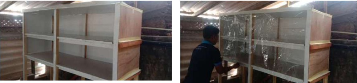
Figure 3: Wooden rack designed for growing algae
