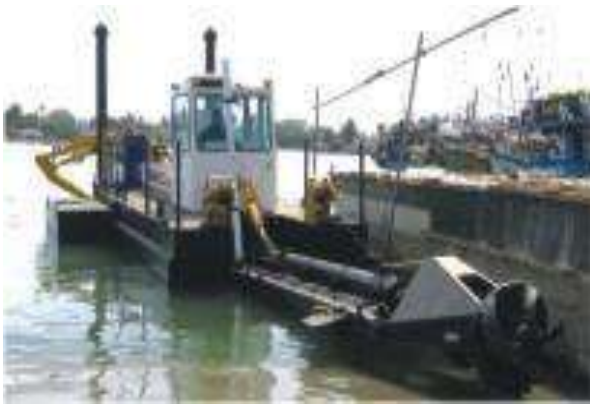
Salapura Kinduri Cutter Suction Dredger
